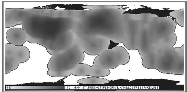
Fig. 6. Theoretical free space loss [dB].
